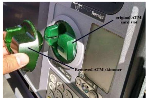
Fig. 1 Skimming device found on an ATM [2]
